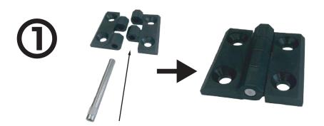
To attach the bases on your Hanoucar, insert the metal rod (serrated side at the end of the stroke) into the aligned notches of the brackets using a hammer.
